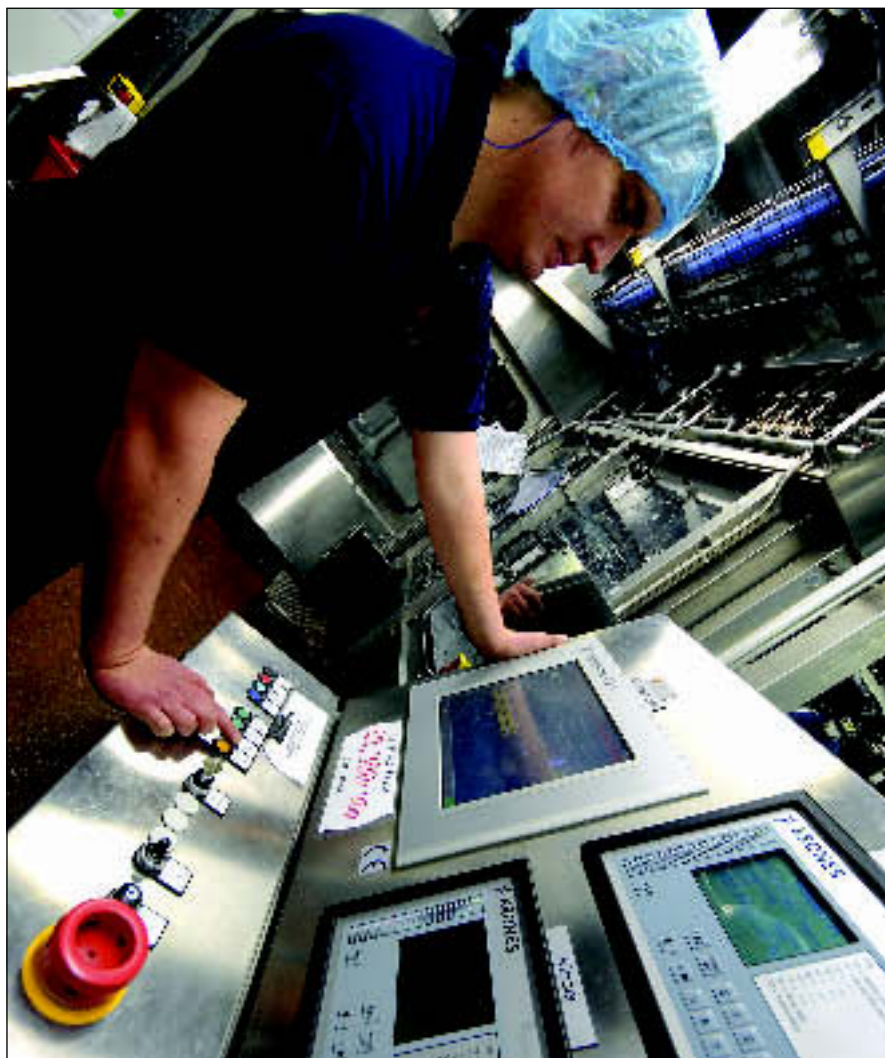
► Control panel of the Kronos PET-Asept filling line which is being used for both Ribena and Lucozade Sport
