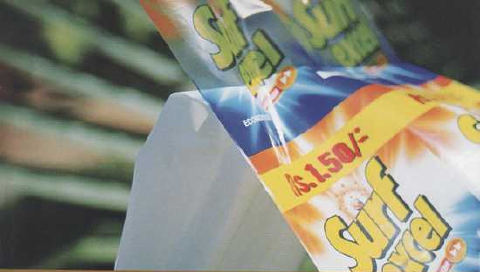
Above 2 (A) laminate for delirigent packaging. Our white opaque PE film, laminated as the support layer to a reverse printed PET film, for excellent fuel-through-contaminator
