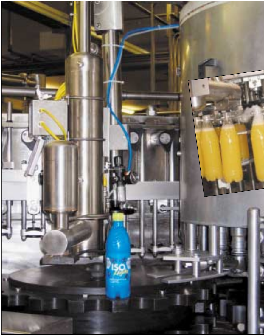
Left: liquid nitrogen injection systems are popular with PET bottles to enable lightweighting to reduce material costs. Left: doser in action — the growing juice, water and flavoured water markets created a boom in demand for its systems says Vacuum Barrier. Top: The bottle on the left was filled using a liquid nitrogen doser, whereas the one on the right didn't and lacked rigidity. Above: the precise nitrogen stream of a dosing head
