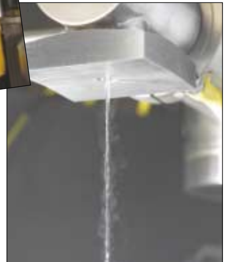
Left: liquid nitrogen injection systems are popular with PET bottles to enable lightweighting to reduce material costs. Left: doser in action — the growing juice, water and flavoured water markets created a boom in demand for its systems says Vacuum Barrier. Top: The bottle on the left was filled using a liquid nitrogen doser, whereas the one on the right didn't and lacked rigidity. Above: the precise nitrogen stream of a dosing head
